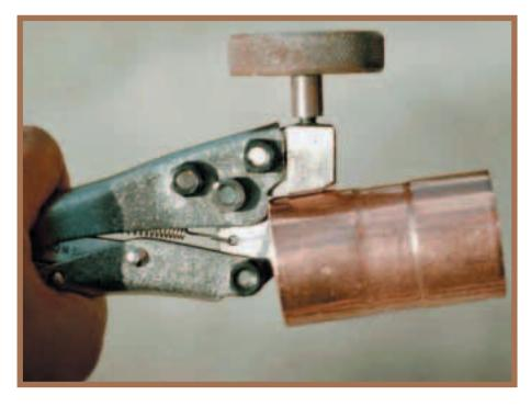
This tool modifies copper fittings by  $_3$  making a shallow impression in the fitting wall, shortening the socket depth to  $\frac{1}{8}$  in. It should be used only for joints that will be brazed.
